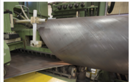
Edge preparation and presentation are just as critical in spiral welding for pipe as they are for any other welding process. As part of its quality improvement plan, Trinity installed laser-based measuring devices that help to eliminate human error.
